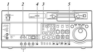
Audio recording level control knobs
